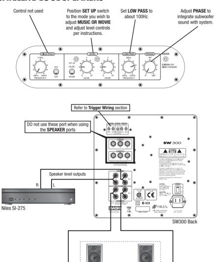
Figure 5. Speaker level connections
